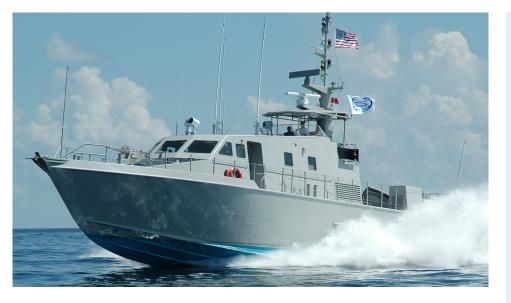
Swiftships' 26 Meter Patrol Craft is a triple water jet, diesel powered, all-welded aluminum patrol craft.
