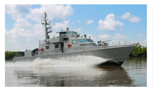
The 35 Meter Patrol Boat hull and superstructure are constructed of all-welded aluminum alloy.
