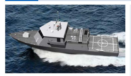
Swiftships' Fast Missile Boat (FMB) hull and superstructure are constructed of all-welded aluminum alloy.
